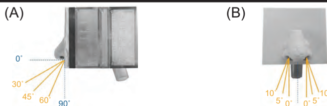
Figure 3. (A) Schematics showing the different configurations tested by varying the horizontal plane angle and (B) vertical plane angle from the center wall.
